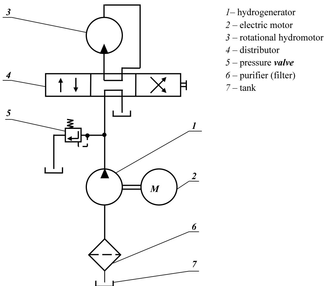
*Hydrogenerator* transfers the mechanical energy of the electric motor to pressure energy using liquids.
