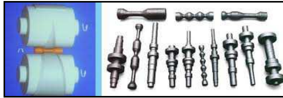
Picture 2 - Cross-wedge rolling with examples of rolled products
